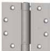
NFPA 80 has restricted the use of architectural grade spring hinges to fire rated doors of a maximum size of 3'0" x 7'0" (914 mm x 2134 mm). Hager spring hinges have been tested and labeled for up to a 4'0" x 8'0" (1219 mm x 2438 mm) door when a minimum of three springs are used. Spring hinges must be used with ball bearing hinges. Do not use plain bearing hinges with spring hinges.
