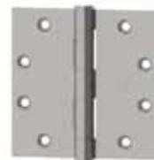
The **Non-Removable Pin (NRP)** has a small set screw in the body of the barrel. This set screw is tightened down against the pin. The pin has a groove in the position where the set screw makes contact, allowing the set screw to seat. The set screw is positioned so it cannot be reached unless the door is opened. If pin removal is necessary, the set screw is merely removed and the pin tapped from the bottom in the usual manner.
