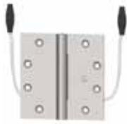
One other product that can be used for a power transfer hinge is an air or pneumatic transfer hinge. This is used to transfer as much as 120 pounds of air pressure through the hinge in order to operate an air modified lock or exit device. Pneumatic power may be used in explosion-proof areas or where electric power is not sufficient to perform the necessary job.
