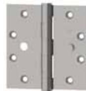
The **Safety Stud (SH)** 3/16" (4.8 mm) projection is a feature that places a stud on one leaf and a locking hole on the other leaf. When the door is closed, the stud is anchored into the opposite leaf. Even if the hinge pin is removed, the door is secure because the leaves are locked together.
