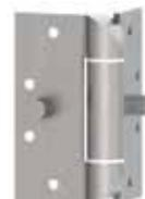
The **Reverse Security Stud (RSS)** 7/16" (11.1 mm) projection is a feature that has a stud projecting from the back of both leaves into the reinforcing plate of both the frame and the door. It is intended to keep the hinge locked in place from abuse of battering or trying to shear the hinge and screws. This feature is primarily used in prisons and psychiatric areas.
